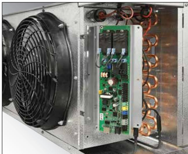
The Master Controller Reverse Cycle Defrost control board is factory installed inside the evaporator coil with an easy to use interface mounted on the outside. The coil features a removable side panel for access to the control board.
